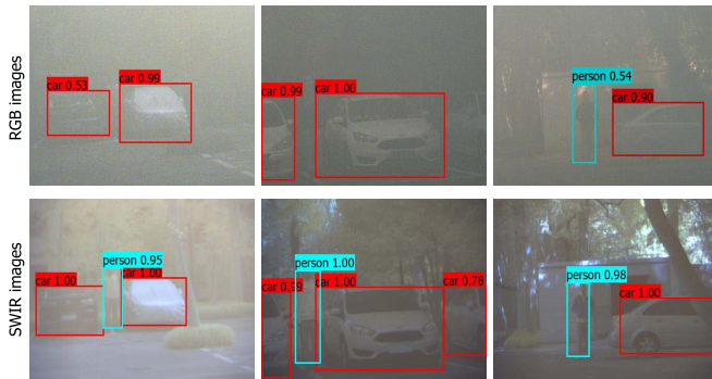
Fig. 1. RGB and SWIR images of haze scenes acquired by our imaging system. The detected pedestrians and vehicles are marked with bounding boxes and confidence scores. Compared with the RGB images, the SWIR images are more clear and produce higher object detection precision.
